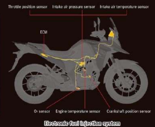
Electronic fuel injection system
