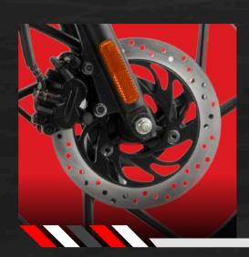
Gear up for quicker braking on any surface with 240 mm ventilated front disc brake along with anti-skid technology. A 1320 mm wheelbase and tubeless tyres ensure further stability.
